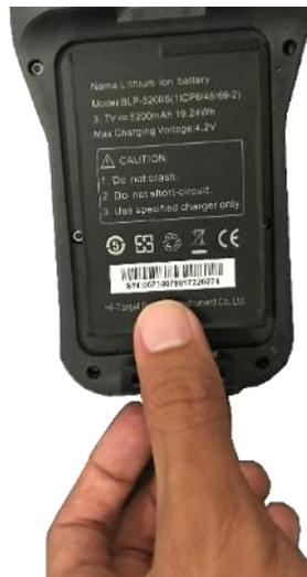
*Figure 5-4-3 Installation of the battery*
