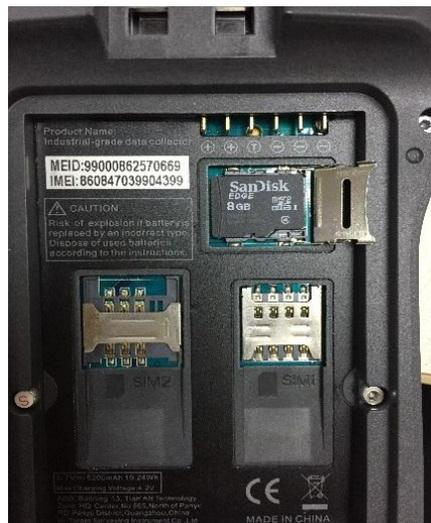
Figure 5-4-14 Installation of Micro SD card
