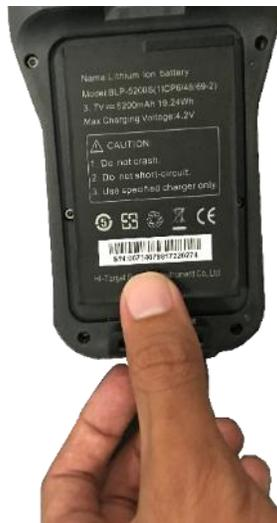
*Figure 5-4-3 Installation of the battery*
