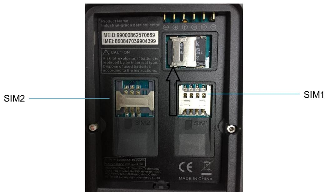
Figure 5-4-9 Installation of SIM card
