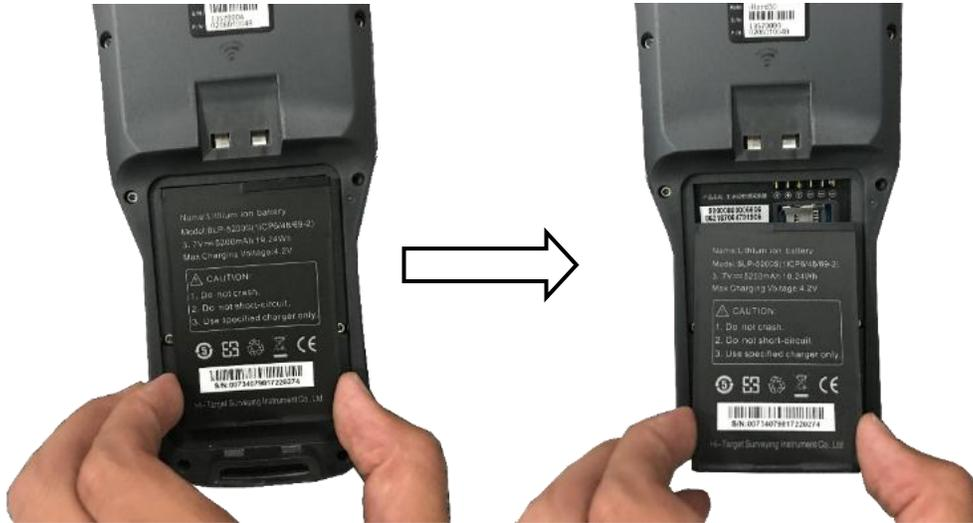
Figure 5-4-4 Dis-assembly of the battery
