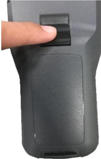
Figure 5-4-6 Lock the battery cover
