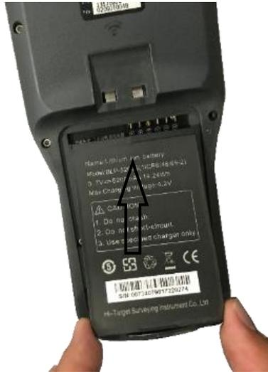
*Figure 5-4-2 Installation of Battery*
