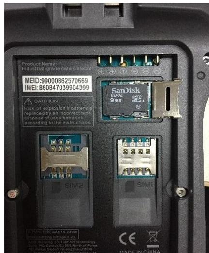
Figure 5-4-14 Installation of Micro SD card
