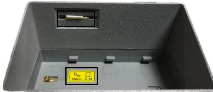
*Figure 4-1-1 SIM card installation*
